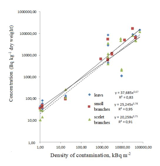
The concentrations of <sup>90</sup>Sr in air-dry matter of plants were increased with increasing soil contamination density in accordance with the exponential dependence.
